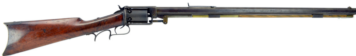
The “Warner Solid Frame Revolving Rifle” of 1851 is depicted above, fitted with a traditional percussion cap system and a manually-rotated cylinder. The tiny spur in front of the trigger unlatches the cylinder for rotation. The ramrods are removed to work the loading lever.
