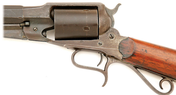
Close-up of a .44 rimfire cartridge conversion
