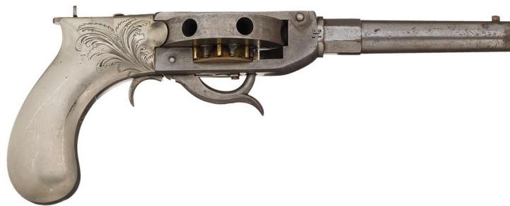
The Cochran “Third Type” Pistol, which nicely reveals the turret mechanism
